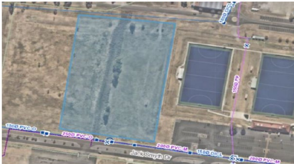
Figure 19 Tamworth Council Existing Water mains
